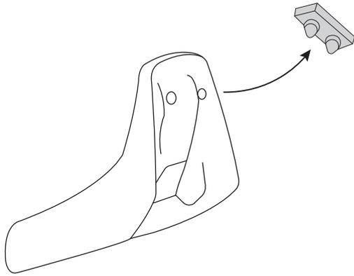
**Remove the original seat and side panels. Remove from the seat the original gasket.**
