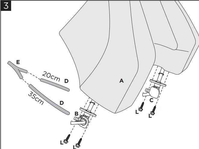
**3** Insert the taps (B) and (C) into the Acerbis fuel tank (A) using the screws (L). Rest the tank on the frame and connect the taps to carburetor through the fitting (E) and the rubber tube (D), cut in the measurements indicated in the figure.
