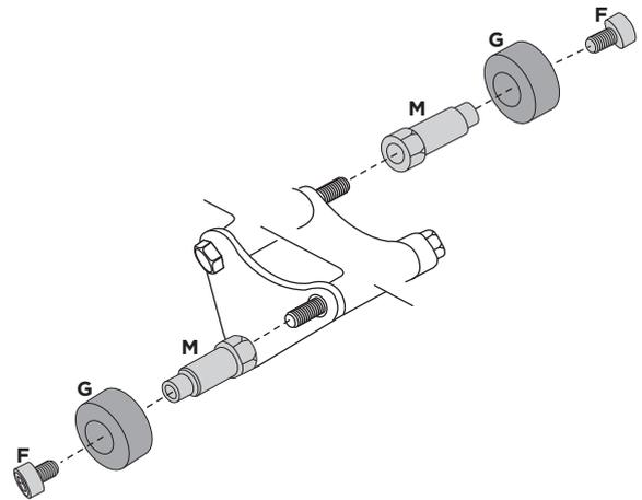
**Take off the original self locking nuts and tighten the bearings (M), with the grommets (G) and the screws (D).**
