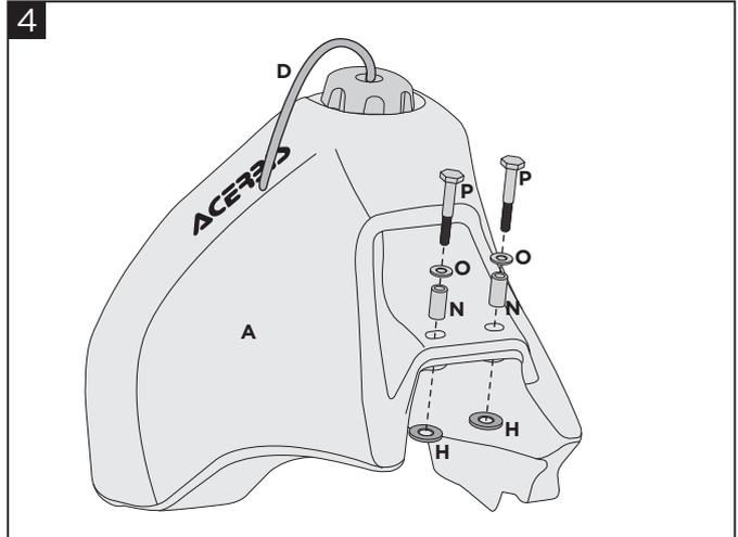
**4** Fix the Acerbis fuel tank (A) to the frame using the screws (P), the washers (O), the spacers (N) and the gaskets (H). Screw the cap with the rubber tube (D). Remount the seat and the original side panels.
